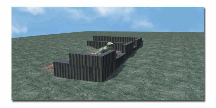
Even temporary observation points can be set up with RESCO Protection Blocks. Since no binders are required for the construction, the observation point can also be easily removed.
